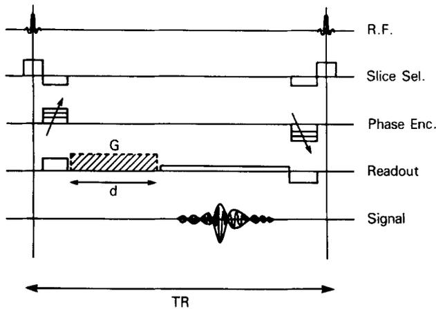
FIG. 1. Diagram of the pulse program used for IVIM-SSFP imaging. The SSFP sequence is sensitized to IVIMs by an additional gradient pulse (strength  $G$ , duration  $d$ ). IVIM images are generated from twin sequences differing only by the presence or absence of the gradient  $G$ .
